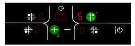
The adjusted zone will continue to operate at the desired setting by getting on and off at varying intervals according to its level.
