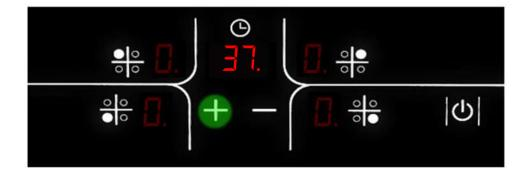
By pressing the button of the zone you want to open (" $\Rightarrow$ ", " $\Rightarrow$ ", " $\Rightarrow$ ", " $\Rightarrow$ "), the setting of that zone is changed and the zone is adjusted to the desired level with the "+" - " -" buttons.
